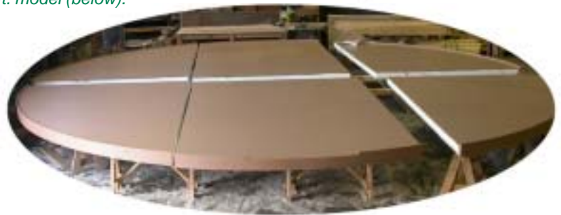
A 10-piece sectional yurt floor for a 28ft. model (above) and a six piece sectional floor for a 20ft. or 24ft. model (below).
